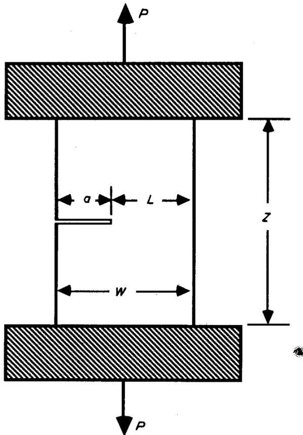
Figure 3 Specimen configuration:  $Z = 80$  mm,  $W = 25$  mm.
