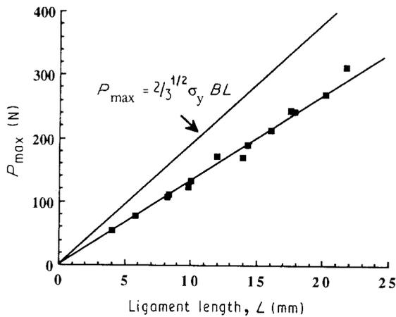
Figure 11 Maximum load as a function of ligament length for K200 ( $B = 0.265$  mm).
