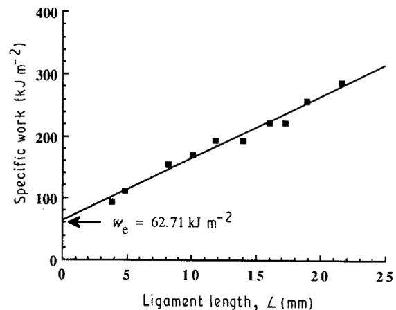
Figure 5 The specific work of fracture for K200 as a function of the ligament length ( $B = 0.250$  mm). The line drawn is the best fit with the equation  $w_f = 62.71 + 10.09 L$ .
