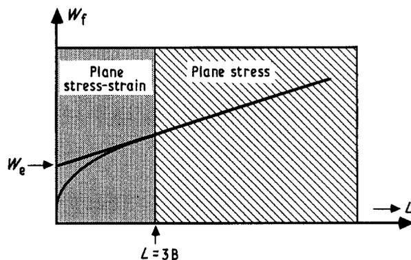
Figure 2 Schematic representation of the total specific fracture work versus ligament length showing plane stress and plane stress-strain regions.
