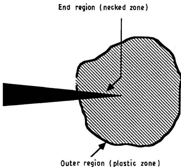
Figure 1 Crack tip deformation zone in a ductile material.
