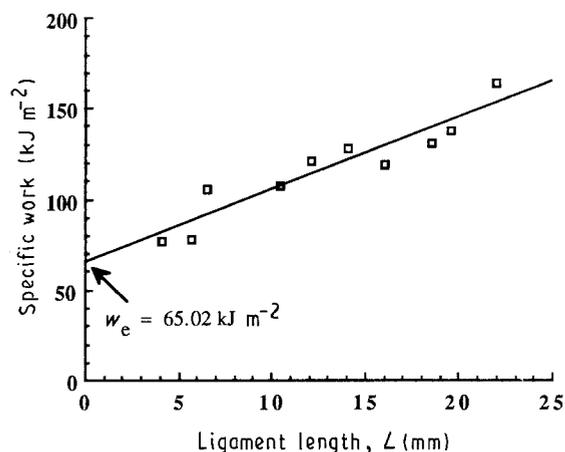
Figure 7 The specific work of fracture for XK300 as a function of the ligament length ( $B = 0.1$  mm). The line drawn is the best fit with the equation  $w_f = 65.02 + 4.0 L$ .
