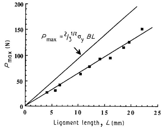
Figure 13 Maximum load as a function of ligament length for XK300 ( $B = 0.1$  mm).
