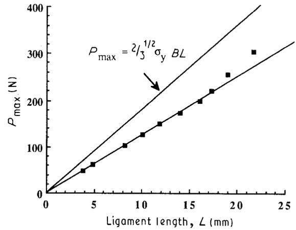
Figure 12 Maximum load as a function of ligament length for K200 ( $B = 0.25$  mm).
