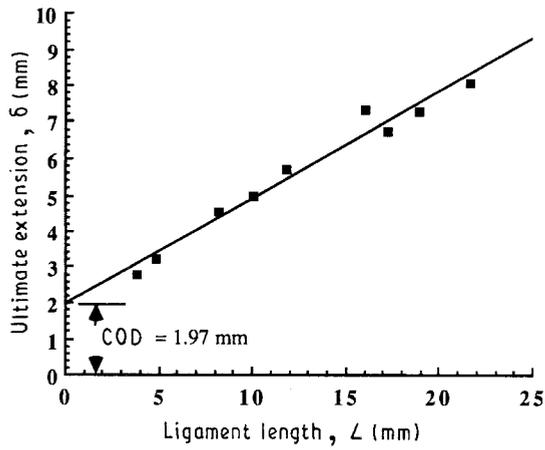
Figure 9 Ultimate extension against ligament length for K200 ( $B = 0.25$  mm). The line drawn is the best fit with equation:  $\delta = 1.97 + 0.29 L$ .
