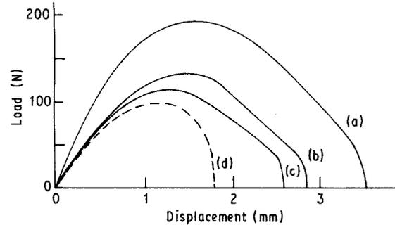
Figure 4 Typical load–displacement curves for (—) K200 ( $B = 0.265$  mm) and (---) XK300 ( $B = 0.1$  mm).  $L$ : (a) 14.26 mm, (b) 11.96 mm, (c) 10.01 mm, (d) 8.32 mm (e) 16.07 mm.
