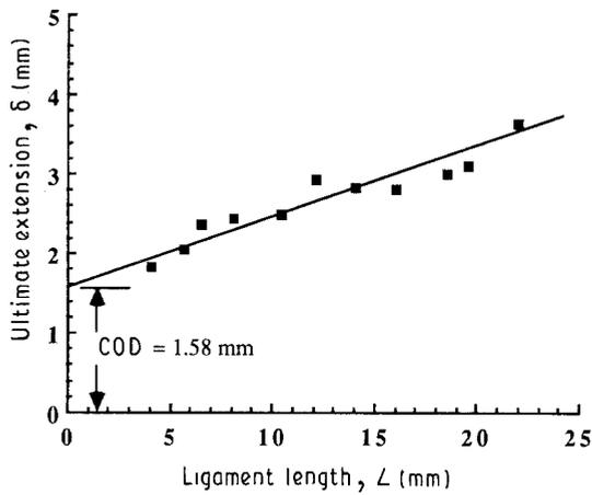
Figure 10 Ultimate extension against ligament length for XK300 ( $B = 0.1$  mm). The line drawn is the best fit with the equation:  $\delta = 1.587 + 0.092 L$ .
