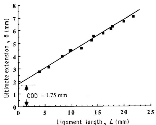
Figure 8 Ultimate extension against ligament length for K200 ( $B = 0.265$  mm). The line drawn is the best fit with the equation  $\delta = 1.75 + 0.258 L$ .
