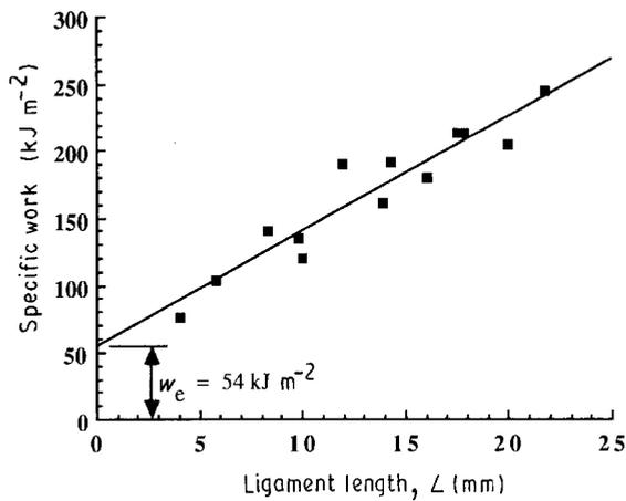
Figure 6 The specific work of fracture K200 as a function of the ligament length ( $B = 0.265$  mm). The line drawn is the best fit with the equation  $w_f = 54.0 + 8.63 L$ .
